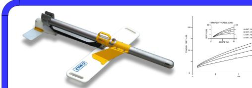
The optional wing depressor pulls the towfish up to 50% deeper. Unlike other depressors the high aspect-ratio wing, with built-in handles, makes for easy launch and recovery. It weighs only 5kg but provides 35kg of downforce at 5 knots.
