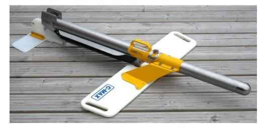
[Note: the design of the CM2 towfish allows a high-aspect-ratio wing to be positioned below the tow point without obstructing the acoustics. This wing and tail combination is significantly more efficient and stable than top-mounted delta-fin depressors.]
