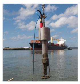
Stema RheoTune in action. Both density and yield stress are measured in-situ without the need of field calibration.
