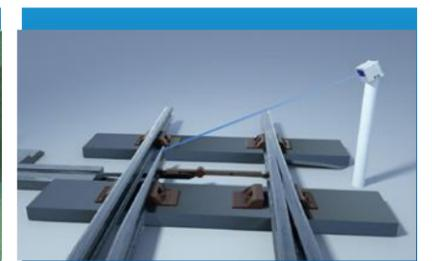
Railway Turnout Deformation Detection Solution
